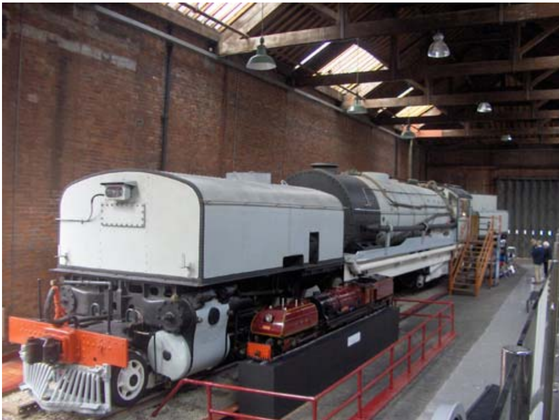
3ft 6inch gauge GL Class Beyer Garratt No 2352 4-8-2 + 2-8-4 works No. 6639 built in 1930
